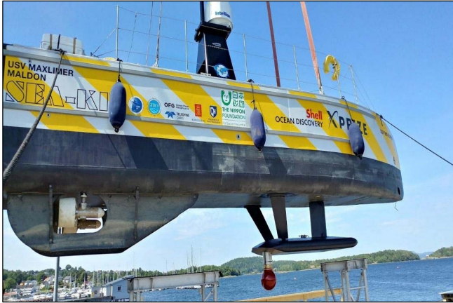
Figure 5. The new gondola installed on SEA-KIT MSV Maxlimer with the HiPAP and multibeam transducers installed. Photo: T. Ketter.
