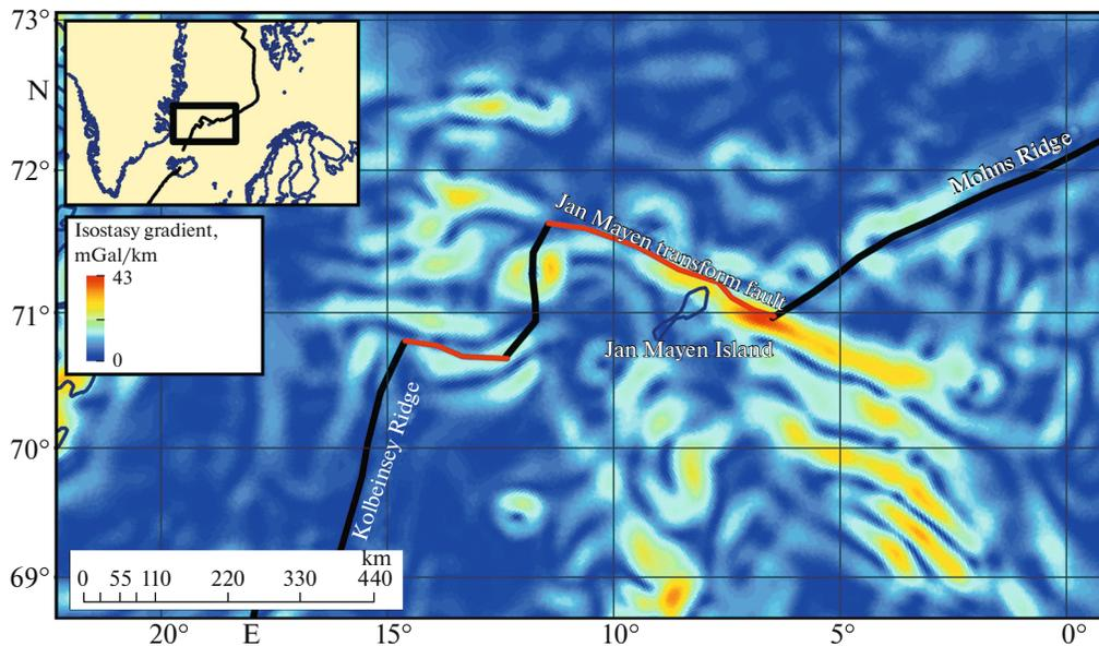
**Fig. 3.** Map of horizontal gradient of isostasy, calculated using the data from [3]. The positions of the main structural elements of the MOR—rift axes (black lines) and transform faults (red lines)—are constructed from the bathymetric data [4].
