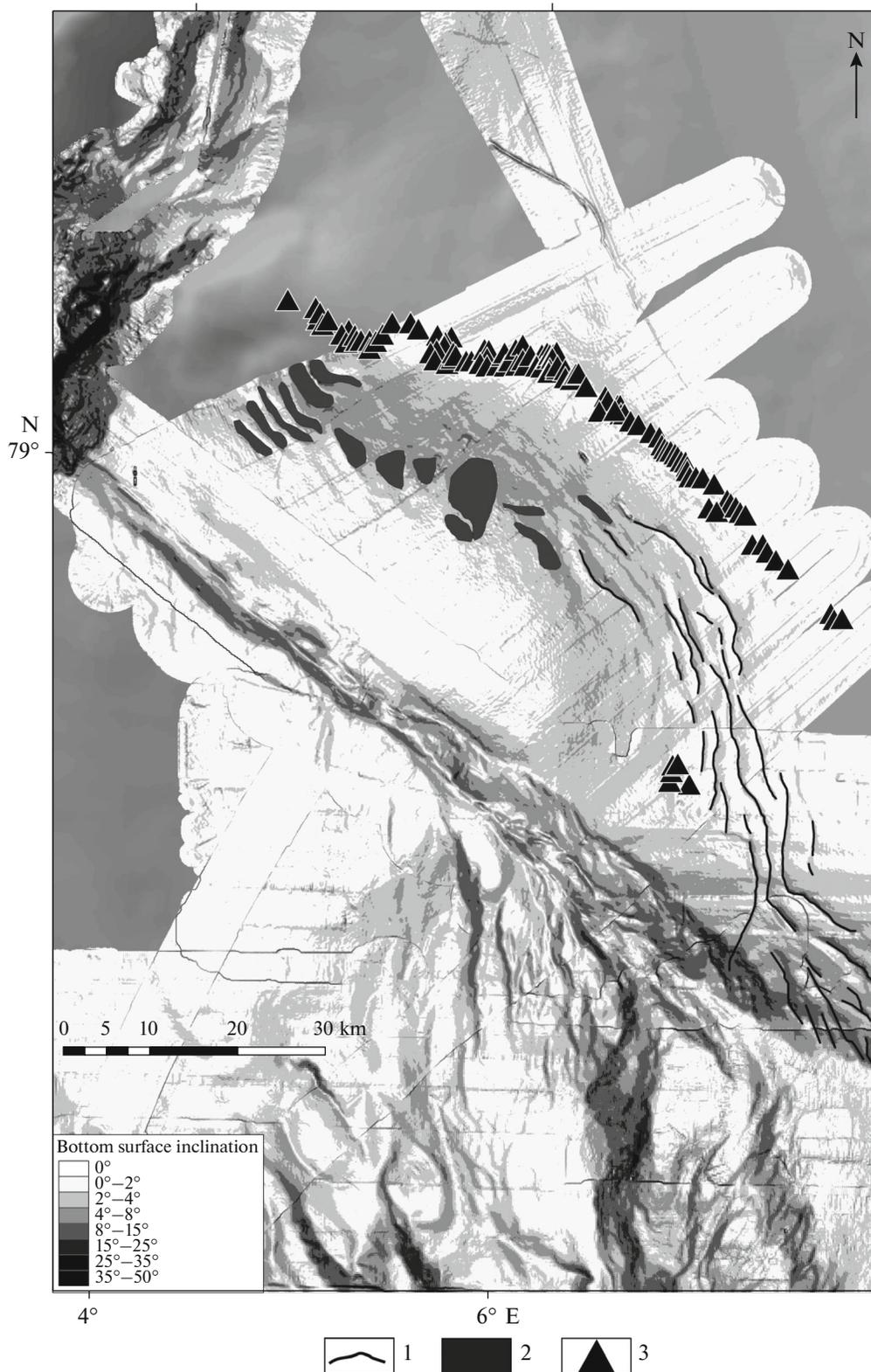
**Fig. 2.** Map of the seafloor inclination (Moroz, 2017). (1) Shrinkage fractures, (2) landslides, (3) gas flares and holes. Topographic base adopted from the data on Cruise 27 of the R/V *Akademik Nikolaj Strakhov* and (Jakobsson et al., 2012).
