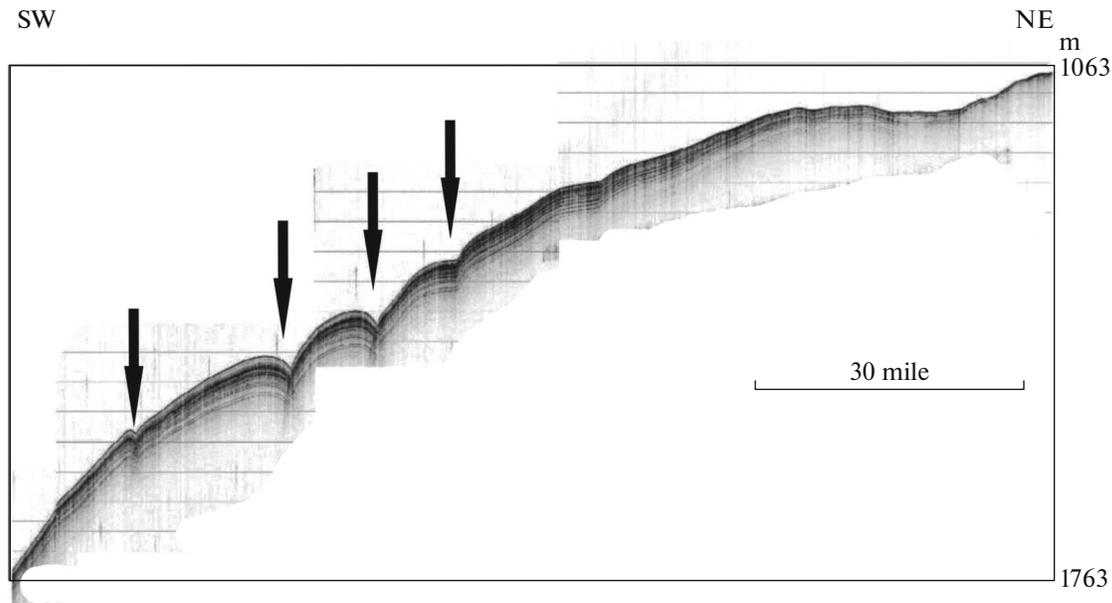
**Fig. 3.** Shrinkage fractures (arrows) on the southern slope of the Vestnesa Ridge (fragment of profile s27-p3-3, Cruise 27 of the R/V *Akademik Nikolaj Strakhov*).
